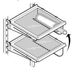
Wine holder can be removed by pulling it straight out and installed by placing it at the end of the shelf you want and pushing it inward.
